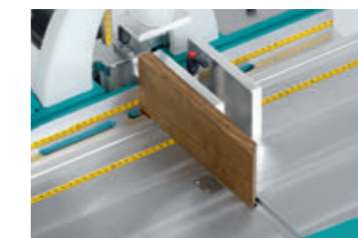
Butt stop fence elevation
