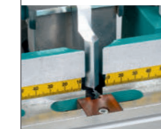
Centre line location jig
