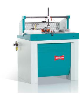
Free-standing version with solid cast table and large working surface at a comfortable working height. With two routing units to produce two dovetail slots in sizes of W-1/2/3 and option W-4. Infinately adjustable router cross-centres from 32 mm to 100 mm.
