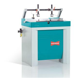
Free-standing version with solid cast table and large working surface at a comfortable working height. With two stations comprising of a single router. Routing two dovetail slots (one in each work-piece) with each machine cycle Hoffmann Key sizes W-1/2/3. Option W-4.
