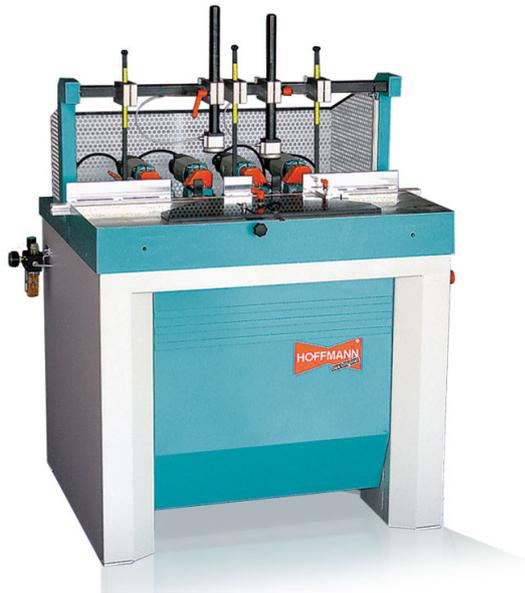
Free-standing version with solid cast table and large working surface at a comfortable working height. With four router units which router two work-pieces on each machine cycle, each with two dovetail slots, for Hoffmann Key sizes W-1/2/3/4. Finely adjustable router spindle centres from 32 mm to 100 mm. When routing cornice profiles the inner and outer sets of routers can be set at different routing heights.
