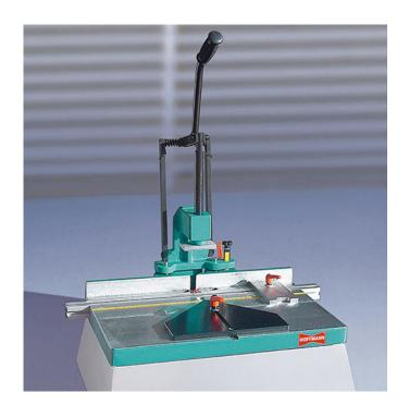
Portable and flexible bench-top machine, for routing a single dovetail slot with each machine cycle. Hoffmann Key sizes W-1/2/3/. Most of the relevant accessories can be used on this machine. Option: Twin version with a double spindle gearbox to produce two dovetail slots per machine cycle.
