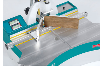
Internal fence elevation
