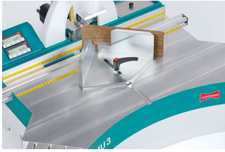
Angle fence plate elevation
